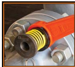
Thread retainer onto stud.
